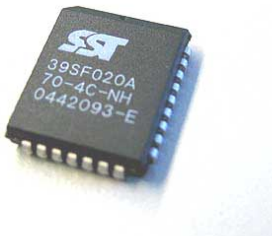
BIOS chip for VIA M10000 mainboard
